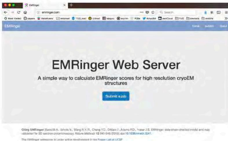
Assesses quality of model-to-map fit of models from cryo-EM using map value interpolation of side chain rotameric positions.
